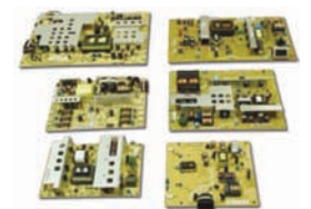
Display Power Supplies
